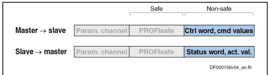
Fig. 3-28: Position of the non-safe process data channel in the cyclic data channel
